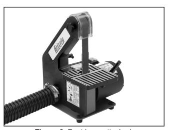
Figure 6. Dust hose attached.
